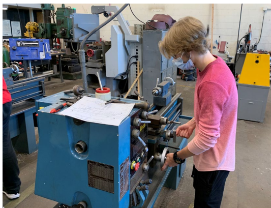
Machining student Greg Williams follows blueprints in using the lathe to shape and cut his project to exact dimensions.
