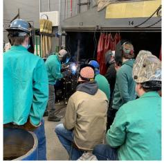
Pictured to the left, Welding Instructor Mr. Joe Villarreal gathers his students to give a specific welding demonstration. Welding is defined by the type of welding that is performed (arc, Tig, Mig, etc.), the type of metal that is being welded, and the position the weld is performed in. In the case of the pictures to the left, Mr. Villarreal is instructing in the following:
