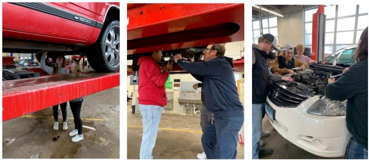
Above: Left- Salina Breckenridge of Putnam County and Olivia Weber of LP track down the cause of engine knocking on a customers truck. Middle- Instructor Mike Fischer (blue) works with Rikki Trinidad of Putnam County to secure a heat and protective shield that has come loose on a vehicle. Right--Miles Walder from PC, Miguel Reveles also PC, Ryker Rolando LP, Rock Ratke LP, and Lincoln Eitutis (back to us) remove head bolts as they prepare to dig deeper into engine of a customers car.
